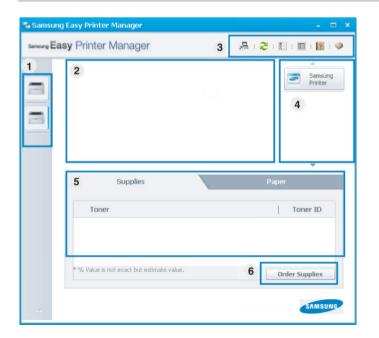
Printer list The Printer List displays printers installed on your computer and network printers added by network discovery (Windows only).
